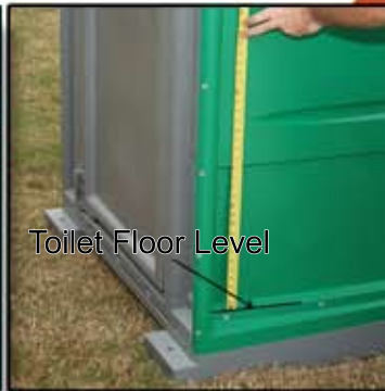
4 Locate holes on the outside of the toilet to align with the holes in the Wash Unit. Drill holes from outside of toilet into wash unit.
