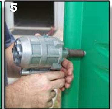
5 Secure Hand Wash Unit in place with supplied rivets
