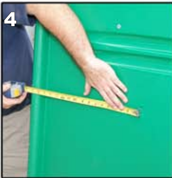
4 Locate holes on the outside of the toilet to align with the holes in the Wash Unit. Drill holes from outside of toilet into wash unit.
