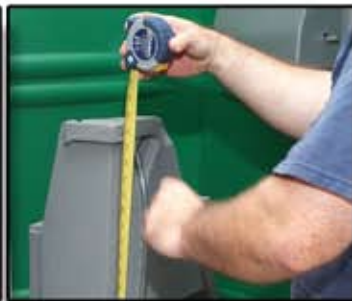
3 Mark and measure holes for rivets on back side of Wash Unit.
